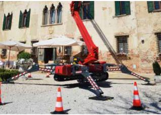
Assisted automatic stabilization on slopes, up to 16°. Allows a ground clearance of 700mm with machine completely stabilized, with slope control during destabilization.
