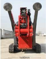
Incredible widening of the undercarriage, from 990mm allowing easy passage through narrow and cramped places, to 1490mm for an enhanced lateral stability.
